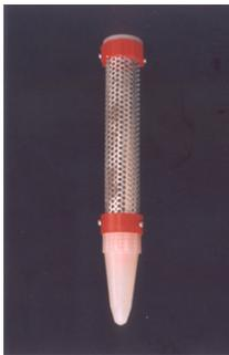
The use of trap is relatively a new method of detecting trapping insects in stored grains. The basic component of a TNAU probe trap consists of three important parts: A main tube, insect trapping tube and a detachable cone at the bottom. Equispaced perforations of 2 mm diameter are made in the main tube.
