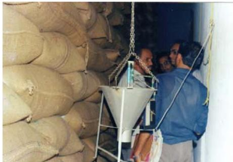
The UV light trap mainly consists of a ultra-violet source (4 W germicidal lamps). The lamp produces ultra-violet rays of peak emission around 250 nano meter. The light is fitted at the centre of a funnel of 310 mm diameter at the top and 35 mm diameter at the bottom. The bottom end of the funnel is attached with a transparent plastic container for collecting the trapped insects. To hang the unit at desired points,
